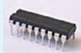
The new 18M2 can now run four separate tasks in parallel, allowing a logicator flowsheet to contain four separate start cells and four separate flowchart tasks. Multitasking is also supported in BASIC program listings. The 18M2 device replaces all of the older 18/18A/18M/18X parts and has memory capacity for up to 1800 lines of code. It is fully backwards compatible with all existing 18 pin PICAXE project boards and programs written for any older 18 pin PICAXE part.
