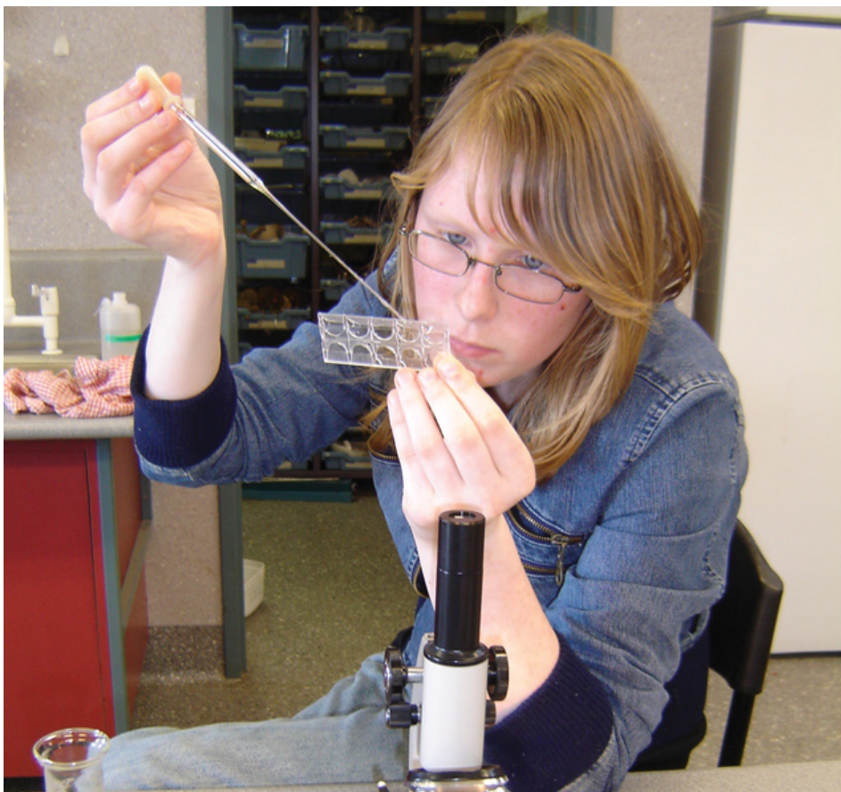
Storm Holwill doing an algae cell count using a haemocytometer
